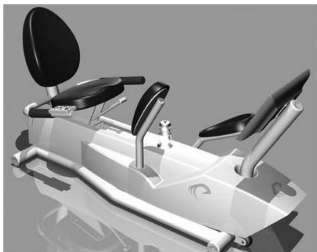
FIGURE 5. An internal motor powers the pedals to move in a reciprocal manner. As the pedal moves towards the participant (to the left in this figure) he or she attempts to slow it down by applying force to the pedal. Because the magnitude of force produced by the motor exceeds that produced by the participant, the pedal continues which results in eccentric lengthening of the quadriceps.
